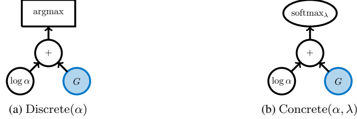
Figure 1: Visualization of sampling graphs for a discrete random variable D \sim \text{Discrete}(\alpha) and a concrete random variable X \sim \text{Concrete}(\alpha, \lambda) . White operations are deterministic, blue are stochastic, circles are continuous, squares discrete. For a single forward pass of the computation every blue node is sampled once; each G_k is sampled via -\log(-\log U_k) where U_k \sim \text{Uniform}(0, 1) i.i.d.; \text{softmax}_\lambda(x) = \exp(x/\lambda) / \sum_i \exp(x_i/\lambda) componentwise for \lambda \in (0, \infty) .
