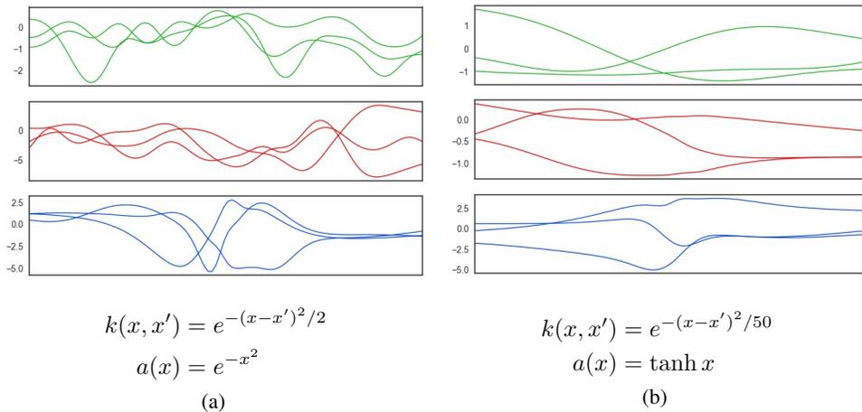
Figure 3: In (a) and (b) we map GP priors with a RBF kernel to BNNs with a RBF and tanh activation functions. It is clear that the optimized samples have taken on the curviness of the GPP samples.
