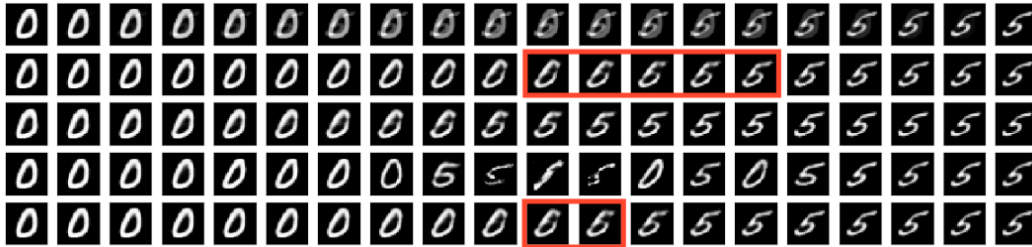
Figure 5: Different interpolations between two MNIST images, represented in the first and in the last column: convex hull in the input space (first row); convex hull between mean vectors, with no sampling (second row); convex hull in the space of the latent variables after sampling of the two images (third row); computation of the geodesics between two Gaussian distributions with sampling along the curve (forth row) and without sampling (fifth row). In red we highlighted the corresponding transition images for the Euclidean and the Riemannian geodesic. The latter geodesic shows a slightly sharper transition.
