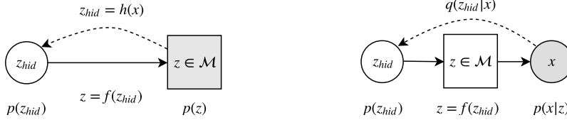
Figure 2: Left: Scheme diagram of WAE with feature space Z and latent space Z_{hid} that learns the prior distribution p(z) on manifold \mathcal{M} \subset Z . Right: The generative model with manifold-valued latent variables z . The squared node is deterministic.
