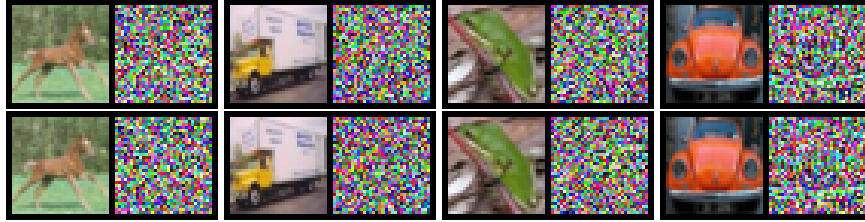
Figure 3: CIFAR-10 test set images and the latent encoding from flow versions of a PixelCNN (top row) and PixelCNN++ (bottom row). We see that certain patterns, such as edges, at times leave footprints in the latent images. While this effect is visible for both models, it is sometimes more pronounced for PixelCNN than PixelCNN++.
