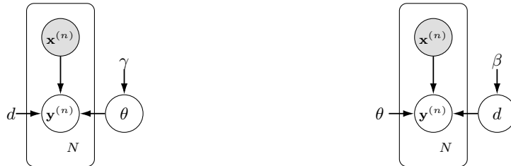
Figure A.2: Left: graphical model of a BNN. Right: graphical model of a DUN.
